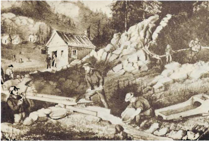
The intensive activity depicted in this 1860 lithograph implies a rich placer area. A canvas water pipe is being used to wash earth (background).
